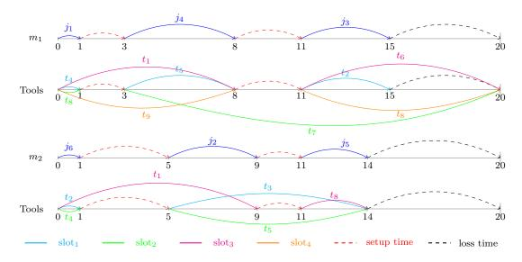
FIG. 2: An AF optimal solution (makespan = 15) of example in Figure 1:
